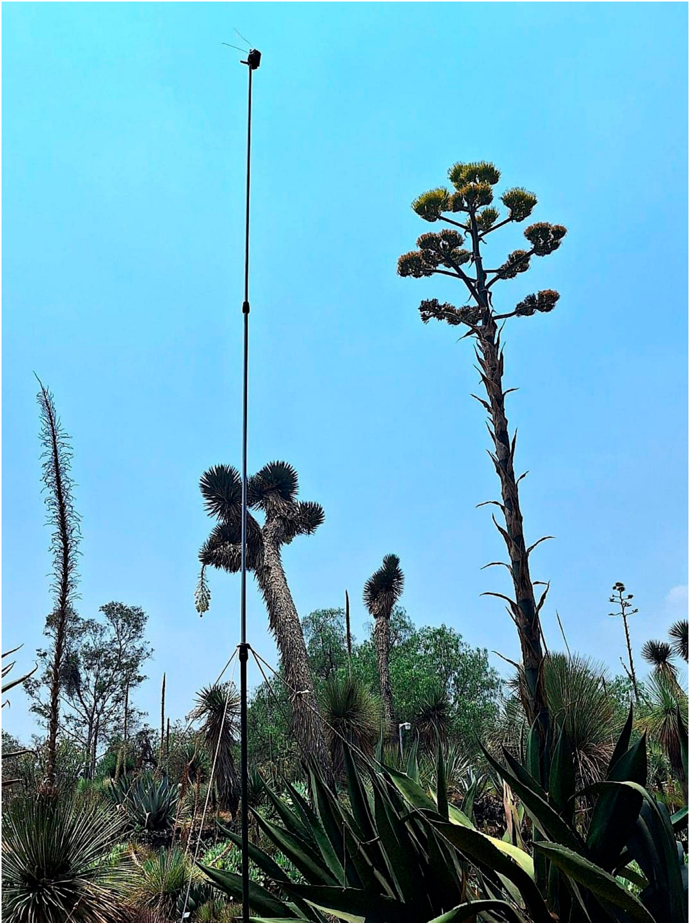
Figure 1. Camera-trap installation used to monitor Agave inflorescences. The camera was mounted on an extendable aluminum pole and stabilized with ropes anchored to the ground, allowing continuous recording of floral visitors on inflorescences located several meters above ground level.
